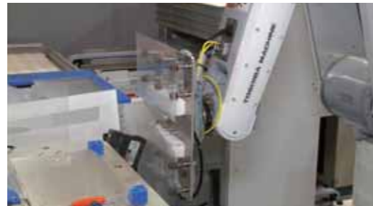
Thickness measurement and appearance inspection of a 10.1-inch thin light guide plate
